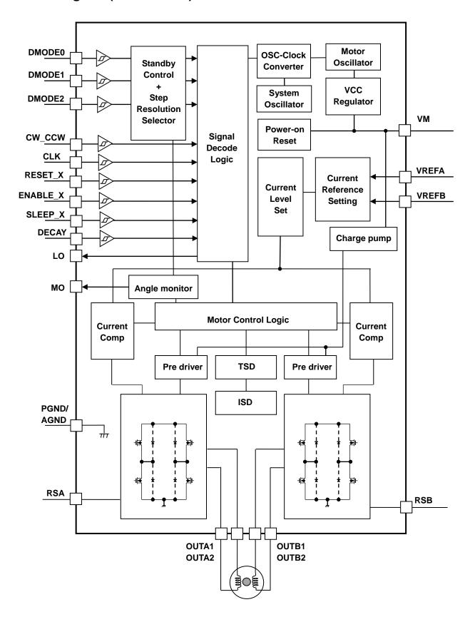
Note: Some of the functional blocks, circuits, or constants in the block diagram may be omitted or simplified for explanatory purpose.
