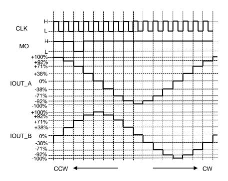
Note: Waveform of MO output: State of pull-up.
