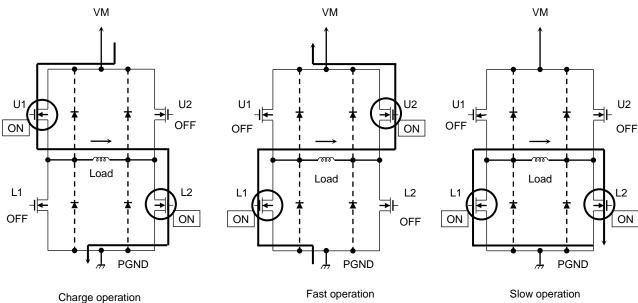
A current flows into the motor coil.
