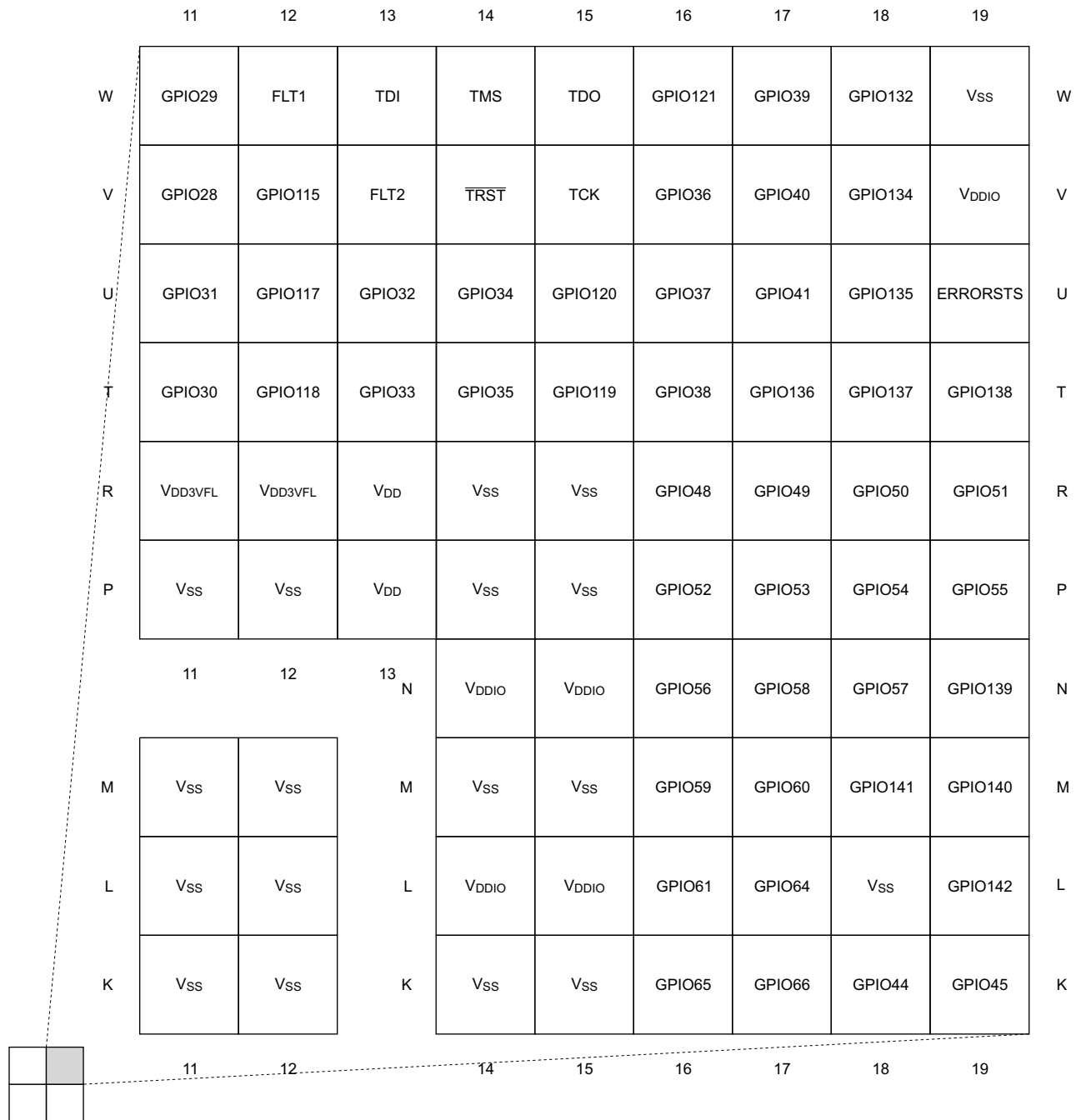
Figure 4-2. 337-Ball ZWT New Fine Pitch Ball Grid Array (Bottom View) – [Quadrant B]
