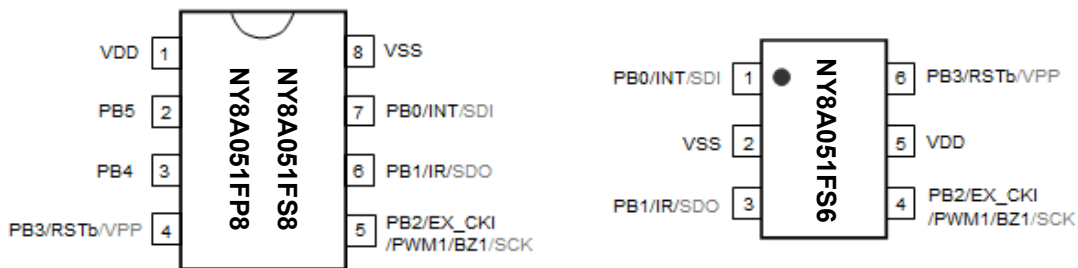
Figure 1 Package pin assignment
