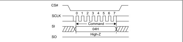
Figure3a. Write Disable Sequence Diagram (QPI)
