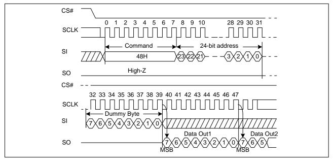
Figure33. Read Security Registers command Sequence Diagram
