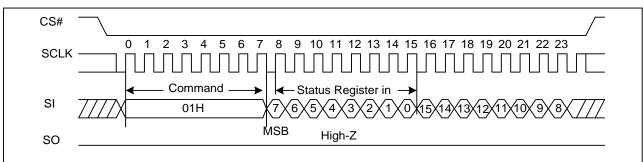
Figure6. Write Status Register Sequence Diagram
