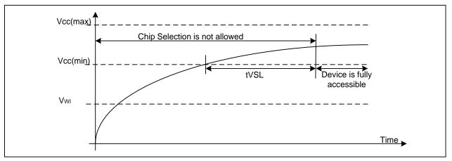
Table6. Power-Up Timing And Write Inhibit Threshold
