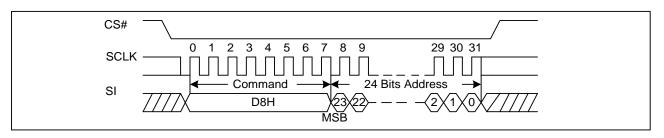
Figure19a. 64KB Block Erase Sequence Diagram (QPI)
