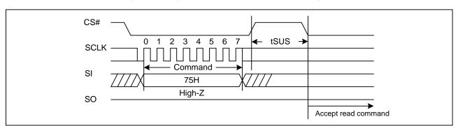
Figure 28. Program/Erase Suspend Sequence Diagram
