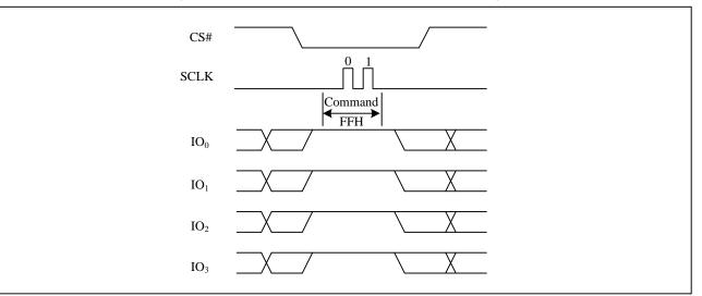
Figure37. Disable QPI mode command Sequence Diagram
