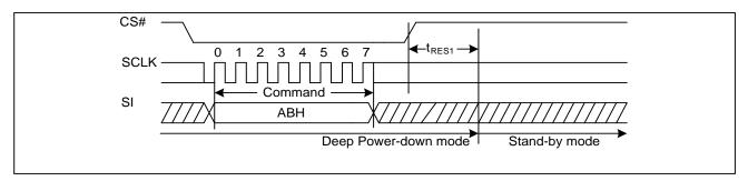
Figure22a. Release Power-Down Sequence Diagram (QPI)
