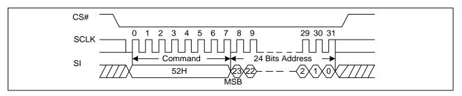
Figure18a. 32KB Block Erase Sequence Diagram (QPI)
