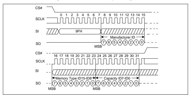
Figure27. Read Identification ID Sequence Diagram
