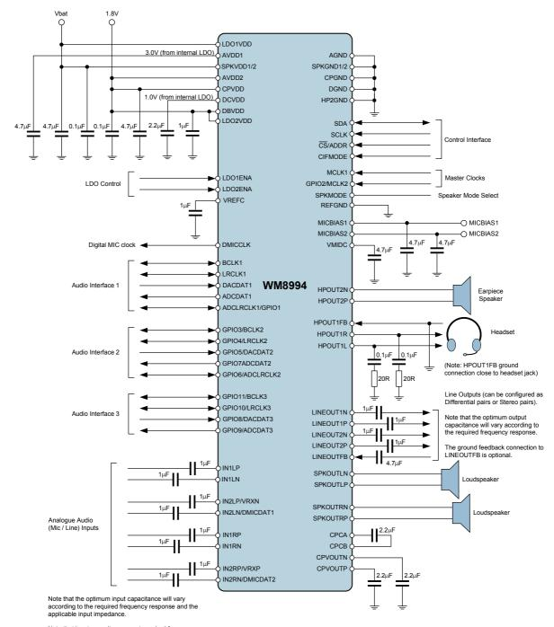
Note that input capacitors are not required for connection to Digital Microphone (DMIC) components
