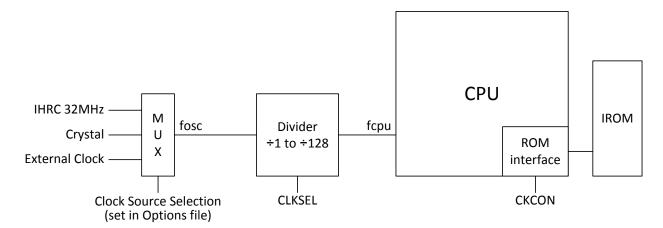
ROM interface is built in between CPU and IROM (program memory). It optionally extends the data fetching cycle in order to support lower speed program memory.
