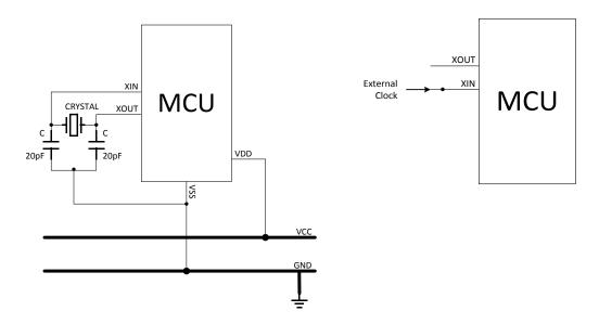
SN8F5703 supplies external low-speed clock ( $f_{RTC}$ ) for the real time clock of Timer 0. In IHRC 32M with RTC mode, the XIN and XOUT pins switch to crystal mode to drive an off-chip 32.768 kHz crystal. The crystal is connected to XIN/XOUT pins with 20pF capacitors to ground.
