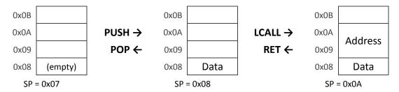
By default, stack pointer (SP register) points to 0x07 which means the stack area begin at IRAM address 0x08. In other word, if a planned stack area is assigned from IRAM address 0xC0, the appropriate SP register is anticipated to set at 0xBF after system reset.
