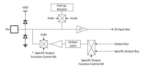
$<sup>{}^{*}.</sup>$  Some specific functions switch I/O direction directly, not through PnM register.
