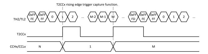
A software split event is triggered by writing any value into CRCL/CCL1/CCL2/CCL3 register. While perform a writing instruction to these registers, the present TH2/TL2 value would be record in the paired registers instead.
