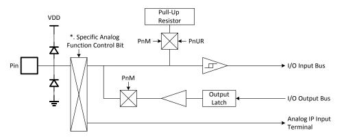
$<sup>{\</sup>bf *}.$  Some specific functions switch I/O direction directly, not through PnM register.
