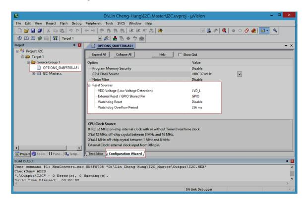
The code option is the system hardware configurations including oscillator type, noise filter option, watchdog timer operation, LVD option, reset pin option and flash ROM security control. The code
