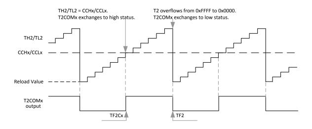
By contrast, the indirectly output method is an event which keep the mapped pin's previous output setting until Timer 2 counter overtakes CRC/CC1/CC2/CC3 register value. In this mode, the transition of the output signal can be configured by software. In other word, the P0.3 register bit would be affect T2COM0/P0.3 pin when TH2/TL2 equal to CRC registers. A Timer 2 overflow causes no output change.
