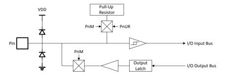
Bi-direction I/O Pin Shared with Specific Digital Input Function, e.g. INT2.
