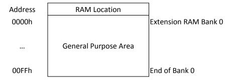
The upper 256-byte XRAM is general purpose RAM and can configure by MOVX instruction access.
