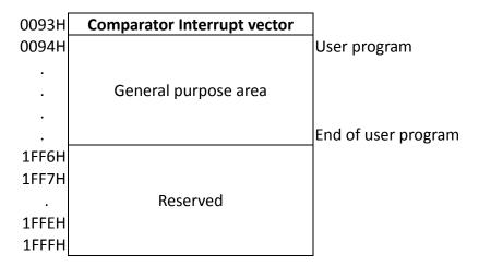
The ROM includes reset vector, Interrupt vector, general purpose area and reserved area. The reset vector is program beginning address. The interrupt vector is the head of interrupt service routine when any interrupt occurring. The general purpose area is main program area including main loop, sub-routines and data table.
