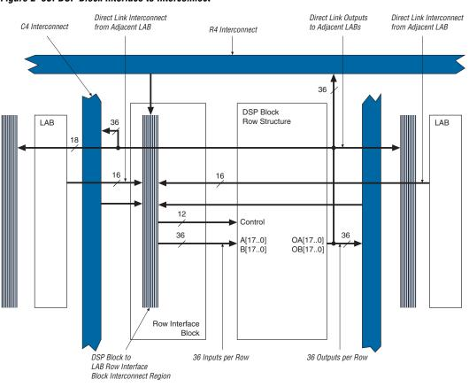
Figure 2–60. DSP Block Interface to Interconnect
