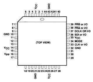
NOTES: A. All pins marked GND are ground connections and must be connected to circuit ground
