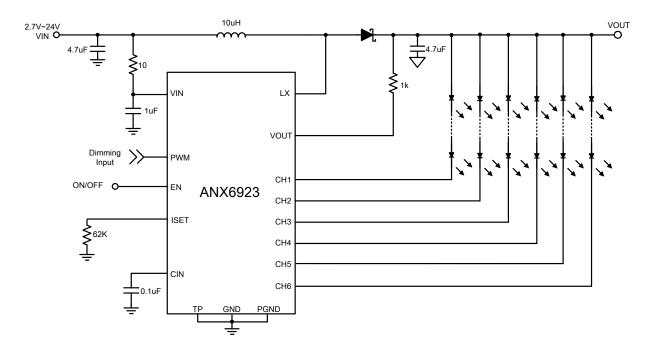
Note1: If the application requires fewer than six LED strings, connecting the unused channels to ground can prevent the boost converter output voltage from temporarily reaching the overvoltage level during power up.
