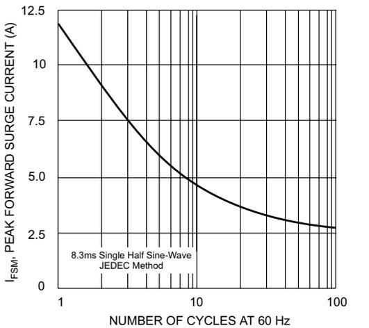
Fig. 3, Maximum Non-Repetitive Peak Forward Surge Current
