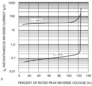
Fig. 4 Typical Reverse Characteristics
