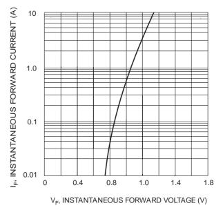
Fig. 2 Typical Forward Characteristics
